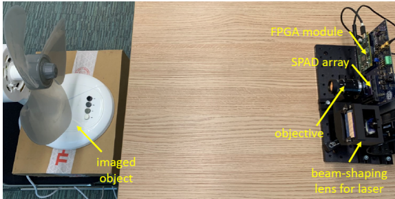
Figure 9. Experimental setup to capture the real SPAD data. The sensor we used here is 192 \times 128 SPAD developed by Henderson et al. [17].
