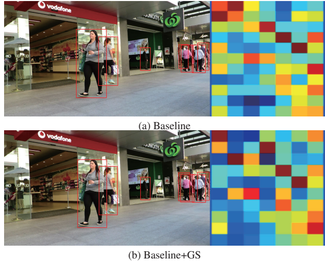
Figure 6. Visualization about the cosine metric matrix between appearance vectors of the current example frame and the track templates. Red color indicates a higher association, and blue indicates a lesser association.
