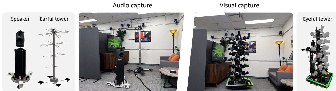
Figure 1. Data capturing setup. (a) Audio capture (left): the loudspeaker and microphone recording system (Earful Tower) are placed at different locations within the room to measure and capture RIRs. (b) Visual capture (right): the camera rig (Eyeful Tower) moves around rooms to capture multi-view images for visual reconstruction and novel-view synthesis.
