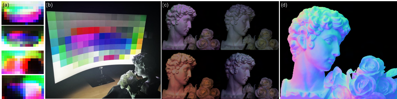
Figure 1. We propose differentiable display photometric stereo, a method that facilitates (a) the learning of display patterns, enabling high-quality reconstruction of surface normals using (b) a monitor and a camera. (c) Capturing a scene with the learned patterns allows for estimating (d) high-quality surface normals.
