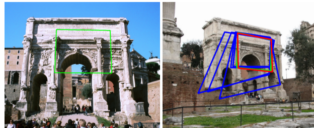
Figure 1. One-point Homography Estimation. A plane from the source image (green patch to the left) is transformed using homographies. Ground truth patch is shown in green in the target image to the right. Blue shows (noisy) transformed patches for the top five inlier samples using the proposed 1-SIFT solver. Red corresponds to the estimated homography resulting from GC-RANSAC [9] with the proposed 1-SIFT solver.
