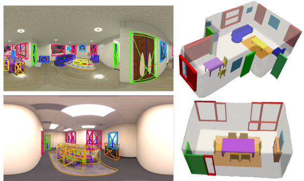
Figure 1. Given a single RGB panorama, we simultaneously estimate the room layout, oriented object bounding boxes (left), and full scene meshes (right). The first and second rows are examples from the iGibson-Synthetic [62] and ReplicaPano datasets.
