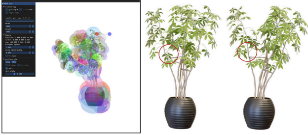
Figure 5. Interactive NeRF deformation. We developed an intuitive UI for users to interact with NeRF scenes like applying external forces and position constraints. Q-GMLS kernels can also be set adaptively to capture local dynamics as highlighted.
