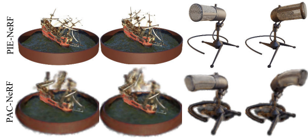
Figure 10. PIE-NeRF vs PAC-NeRF. PAC-NeRF [37] is a closely relevant competitor. A major limitation of PAC-NeRF is the rendering. It is less intuitive to infer the right color/texture information under large deformation using MPM. PIE-NeRF overcomes this limitation with ease. Using implicit time integration, PIE-NeRF runs much faster than PAC-NeRF (two orders in these examples).
