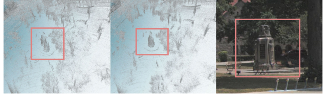
Figure 3. Sequence alignment visualization. The initial GPS-based alignment is imprecise, as evidenced by the duplicated structures in the overlaid LiDAR point clouds (left). After our ICP alignment, the area is well reconstructed (middle) according to its real geometry (right, from Argoverse 2 [61]).
