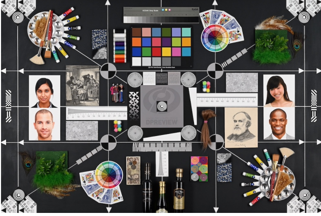
Figure 4. A sample image from the newly proposed DPreview [2] dataset. The presented scene is optimized for camera quality analysis and offers a wide range of colors, textures, and details. The dataset consists of over 294 sensors that capture this scene.
