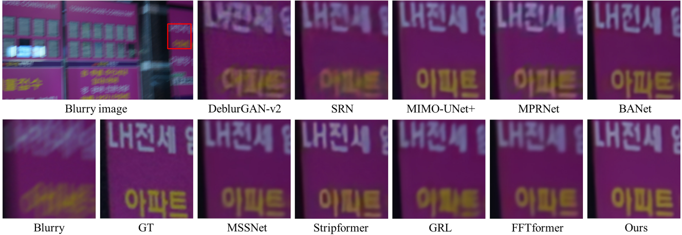
Figure 4. Visual comparisons on the RealBlur-J dataset [23]. The proposed method generates an image with clearer characters.
