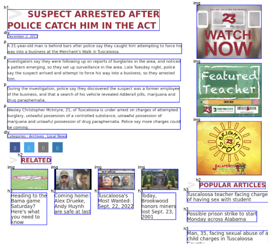
Figure 3. Visualization of layout parsed from a screenshot. Corresponding HTML tags like <h1> are visualize on top-left corner of the bounding box.
