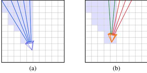
Figure 3. SOAC’s visibility grid (Sec. 3.5). (a) Grid filling: Rays from camera  $C_i$  fill the visibility grid linked to Nerf  $\Theta_i$ . (b) Ray filtering: For cameras  $C_j, \forall j \neq i$ , rays are kept or filtered according to visibility from (a).
