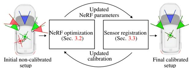
Figure 1. **Method overview.** SOAC is a novel multimodal spatio-temporal calibration method for cameras and LiDAR in the context of autonomous driving. By alternating the training of multiple implicit scenes (Sec. 3.2) and sensors co-registration from these representations (Sec. 3.3), SOAC achieves precise self-supervised calibration from raw data acquired in unconstrained urban environments.
