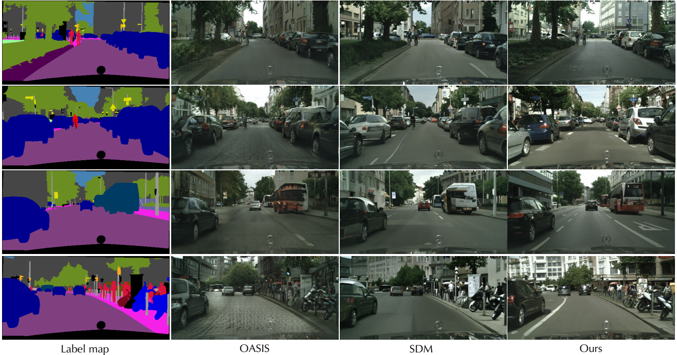
Figure 4. Qualitative comparison with prior work on the Cityscapes dataset. We show the results of OASIS [53], SDM [61], and our approach along with the corresponding label map used for generating each image. Note that our method generates more coherent objects with realistic textures in comparison.
