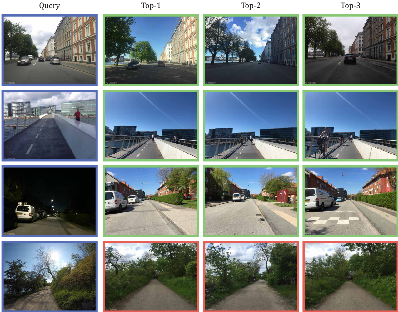
Figure 5. DINOv2 SALAD qualitative results at MSLS. The left column shows several queries and the three other ones shows the top-3 candidates retrieved by our DINOv2 SALAD. Candidates are framed in green if they correspond to the same place as the query, and in red if they do not. Note the correct retrievals under seasonal, weather, viewpoint and day-night changes. Note also a challenging failure case in the last row, due to non-discriminative image content.
