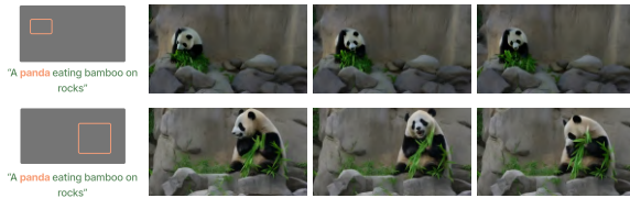
Figure 3. Spatial control with PEEKABOO: Changing the bounding box while providing the same prompt leads to generated panda being faithful to the input layout in terms of size and location with our method.
