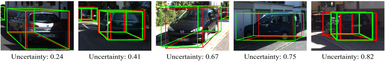
Figure 4. Qualitative illustration of object detection and the corresponding detection uncertainties on KITTI val set. Red boxes denote ground-truth annotations and Green boxes denote our predictions. The detection accuracy is closely correlated with the detection uncertainty. Best viewed with zoom-in.
