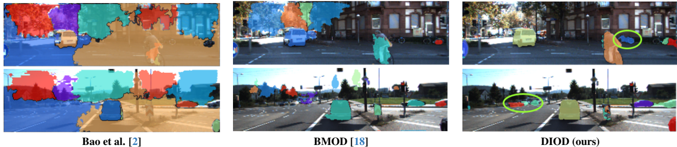
Figure 4. Qualitative comparison of DIOD with previous methods in real-world scenes (KITTI [11]). Each colored mask represents the content of one slot. The green ellipse highlights difficult cases (small or/and static objects) that are correctly segmented in DIOD only.
