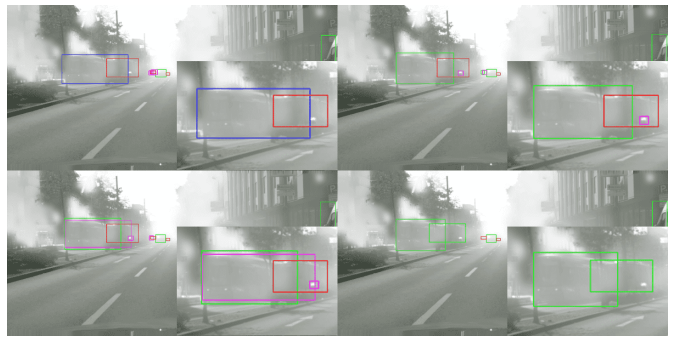
Figure 1. Performance of Class-Aware Teacher (CAT). AT [29] (top left), with Inter-Class Loss, ICL, (top-right), with Class Relation Augmentation, CRA, (bottom-left), and CAT (bottom-right). CAT is able to address misclassification and false positives, blue and red boxes, respectively, in minority classes such as 'train'. The combination of ICL and CRA further boosts performance by reducing the number of false positives shown as pink boxes.
