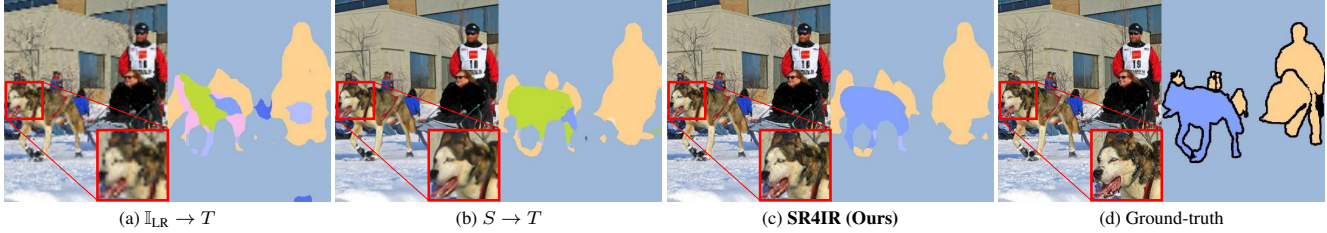
Figure 4. Visualization of images and semantic segmentation results on PASCAL VOC dataset. We present the restored images and the corresponding predicted segmentation maps, respectively. For (b) and (c), we use the SwinIR model with an SR scale factor of x4.
