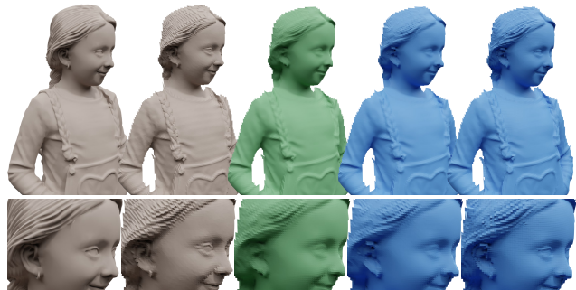
Figure 8. Compared to the usual approach of normal integration using the input image grid, our integration using quadrilaterals on pixels reconstructs a 3D surface with more accurate normals. From left to right: GT mesh that the GT depth map is sampled from, GT depth map, BiNI [5] result, our result with depth averaging per quadrilateral, and our result without the averaging. The last column shows near-identical shading to the GT mesh and depth.
