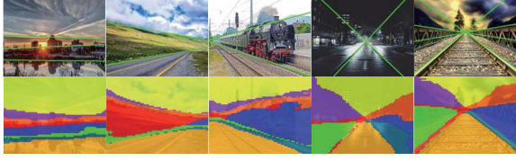
Figure 5. Visualization of semantic feature grouping results. The top row shows input images with ground-truth lines. The bottom one presents the membership maps, representing the semantic region that each pixel belongs to.
