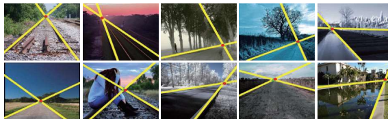
Figure 10. Detected dominant parallel lines and their intersections are depicted by yellow lines and green triangles, respectively. The ground-truth VPs are depicted by red dots.
