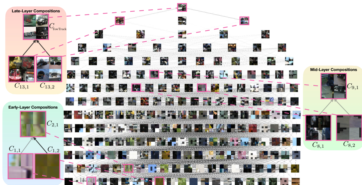
Figure 1. A Visual Concept Connectome (VCC). At each layer the visual concepts learned by a deep model for a given class are revealed as are the learned interlayer concept connections. For each concept, up to four exemplars are shown as unmasked regions in a 2 \times 2 image. Interlayer concept connections are shown as lines with darker lines indicating larger contributions. Shown is a VCC for every convolutional layer of a VGG16 model [49] trained on ImageNet [15] targeting recognition of class “Tow Truck”. A closer visualization of VCC subgraphs reveals interesting compositions occurring at different levels of abstraction corresponding at different depths of the model. At early layers (bottom left), we observe oriented patterns ( C_{1,1} ) and brown color ( C_{1,2} ) composing the concept of green and brown orientation ( C_{2,1} ). Middle layers (right) show the concept of ‘wheel on the road’ ( C_{9,1} ) being composed of wheels ( C_{8,1} ) and regions of asphalt ( C_{8,2} ). The final layer concepts (top left) show that both foreground objects, e.g. tow trucks ( C_{13,1} ), and background regions, e.g. road, trees, humans, or car being towed ( C_{13,2} ), concepts highly influence the final category ( C_{TowTruck} ).
