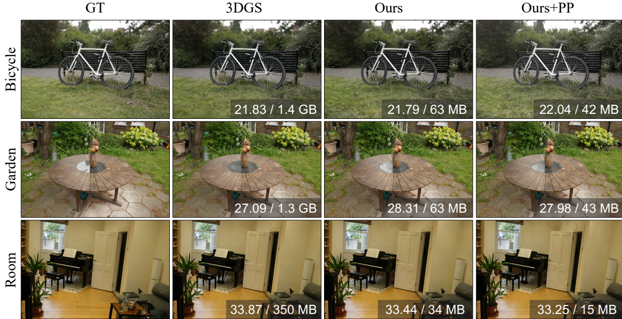
Figure 5. Qualitative results of our approach compared to 3DGS. We present the rendering PSNR and storage on the results.
