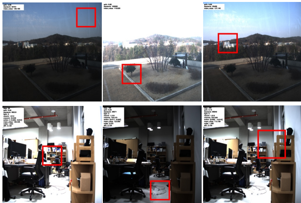
Figure 7. RoI-aware camera exposure control. Our agent is able to control camera exposure for a specific RoI or entire image. Given a RoI box, the agent adjusts the camera parameters to maximize the image attribute for a specific RoI area. It allows the camera to capture the detailed context for the regions of interest.
