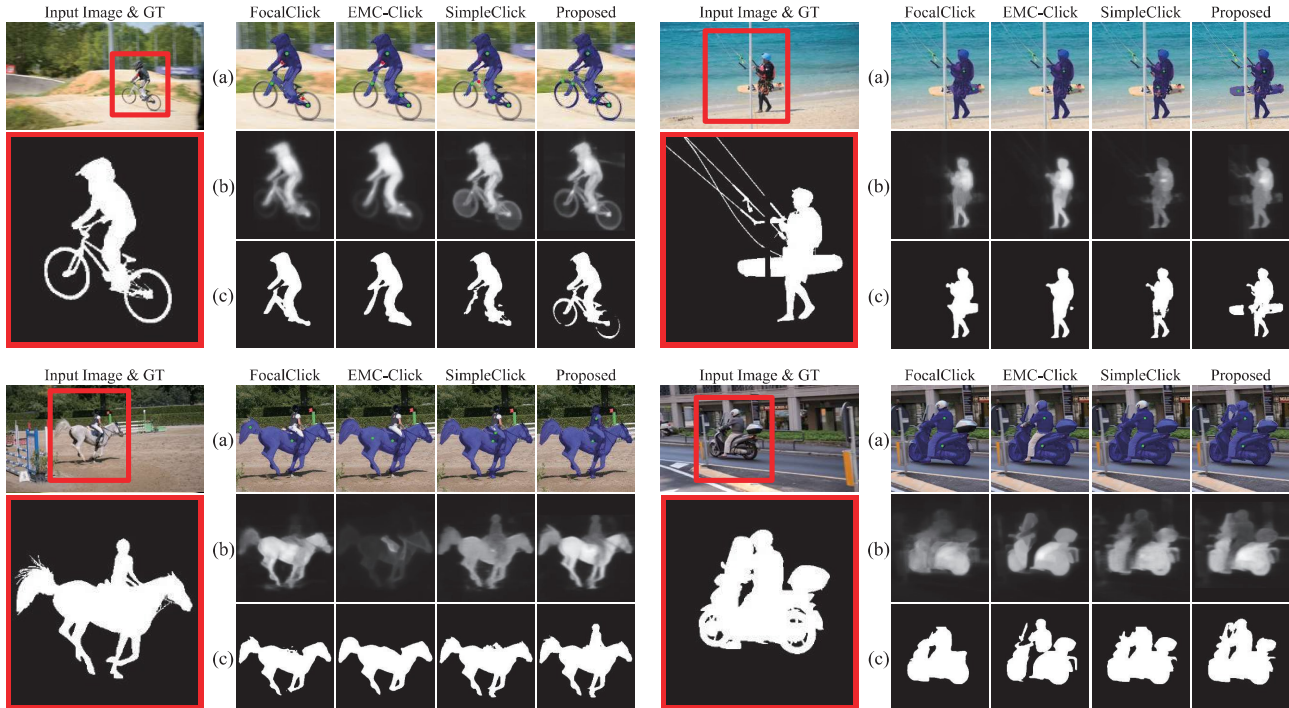
Figure 6. Qualitative comparison of algorithms trained on the COCO+LVIS dataset. We compare the proposed MFP with conventional algorithms that employ previous masks as input: FocalClick [4], EMC-Click [7], and SimpleClick [21]. Rows (a) show input images with clicks and prediction masks overlaid. Rows (b) and (c) show previous probability maps and current prediction masks, respectively. Note that the algorithms are compared fairly using the same automatic clicking strategy. Since the algorithms produce different segmentation results, click locations may differ accordingly.
