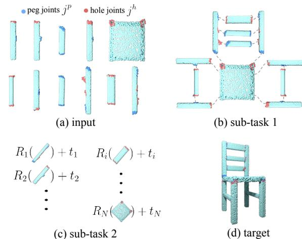
Figure 1. (a) Joint-annotated part point cloud input where blue points indicate peg joints and red points denote hole joints. (b) joint pairing process to produce a bipartite matching between pegs and holes (c) joint-matching-aware SE(3) pose prediction for each part to achieve the target (d) of assembling a shape of a valid structure and with all pegs and holes aligned.
