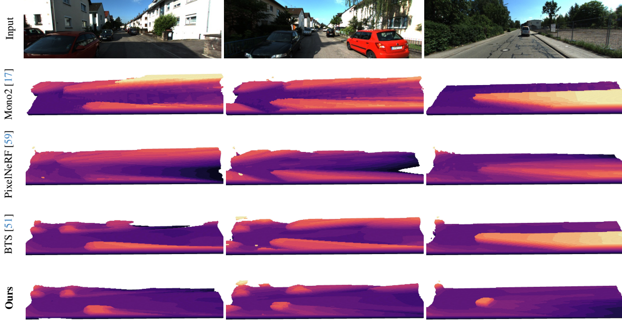
Figure 3. Qualitative comparisons on KITTI-360 dataset. We illustrate the scene reconstructions as voxel grids, where the camera is on the left side and points to the right along the z -axis. A lighter voxel color indicates higher voxel positions. Compared to previous methods that struggle with corrupted and trailing shapes, our method produces faithful scene geometry, especially for occluded areas.
