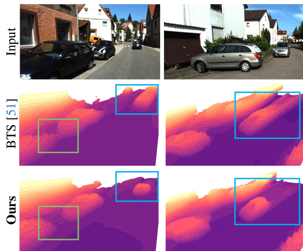
Figure 1. Single-view scene reconstruction results. We present the predicted 3D occupancy grids given a single input image. The camera is at the bottom left and points to the top right along the z -axis. Previous methods like BTS [51] struggle to recover accurate object shapes (green box) and exhibit trailing effects in unobserved areas (blue box). In contrast, KYN recovers more accurate boundaries and mitigates the trailing effects prevalent in prior art.
