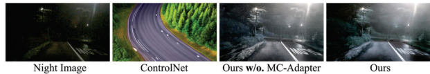
Figure 7. Visual showcase of our LightDiff with and without the Multi-Condition Adapter. The input for ControlNet [55] remains consistent, comprising the same text prompt and depth map. Multi-Condition Adapter makes better color contrast and richer details during enhancement.
