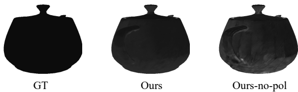
Figure 6. Roughness comparison. Without polarization cues, the recovered roughness is easily affected by geometry and shadows.
