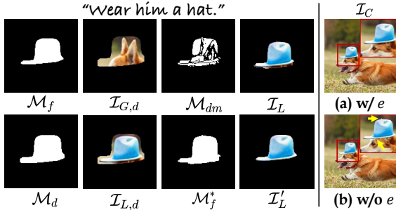
Figure 4. Visualization and ablation. The first 4 columns show the intermediate results related to the edge smoother. The last column compares the final edited results with and without the edge smoother.
