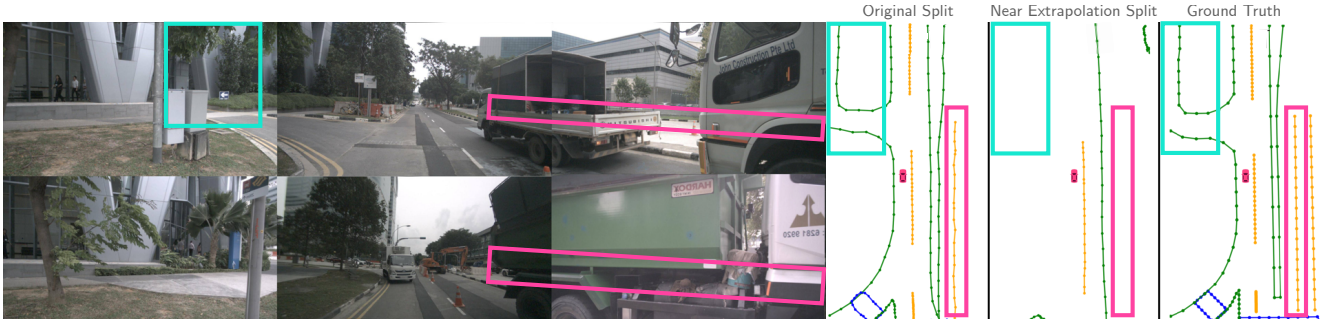
Figure 4. Predictions from MapTR [18] trained on Original and Geographical splits along with the ground truth. Yellow lines denote (lane) dividers, green (road) boundaries, and blue pedestrian crossings. Note that, when trained on the Original split, the branch to the parallel road on the left (teal box) is not visible in any image, yet appears in the predicted map. Also, the divider on the opposing road to the right (pink box) is predicted very well. When training on geographically split data (here Near Extrapolation), this method fails to predict these.
