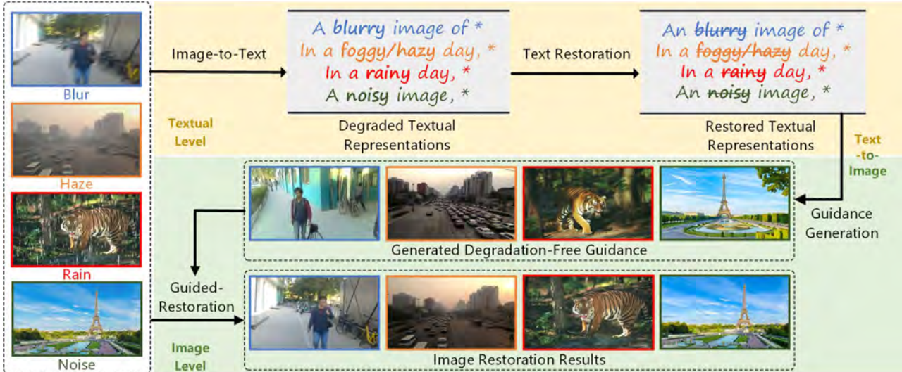
Figure 1. Overview of the proposed method. We propose to improve image restoration by performing restoration on the textual level, in which content and degradation information are loosely coupled. We first encode image concepts into textual space and then remove degradation-related information. To achieve cross-modal assistance, we employ pre-trained T2I models to generate clean guidance for the image restoration process.
