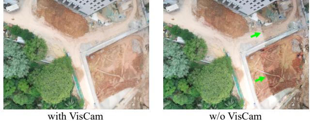
Figure 7. The visibility-based camera selection can eliminate the appearance jumping on the cell boundaries.
