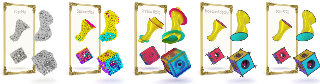
Figure 1. Point2CAD is a pipeline for reconstructing complex CAD models, including freeform surfaces, from 3D point clouds. A raw point cloud is segmented into clusters corresponding to CAD faces, and each face is fitted either with a geometric primitive or with a parametric freeform surface, using a novel, implicit neural representation. Due to the analytic representation the surfaces can be extended and intersected, such that topology emerges, which is then used to clip the surface primitives.
