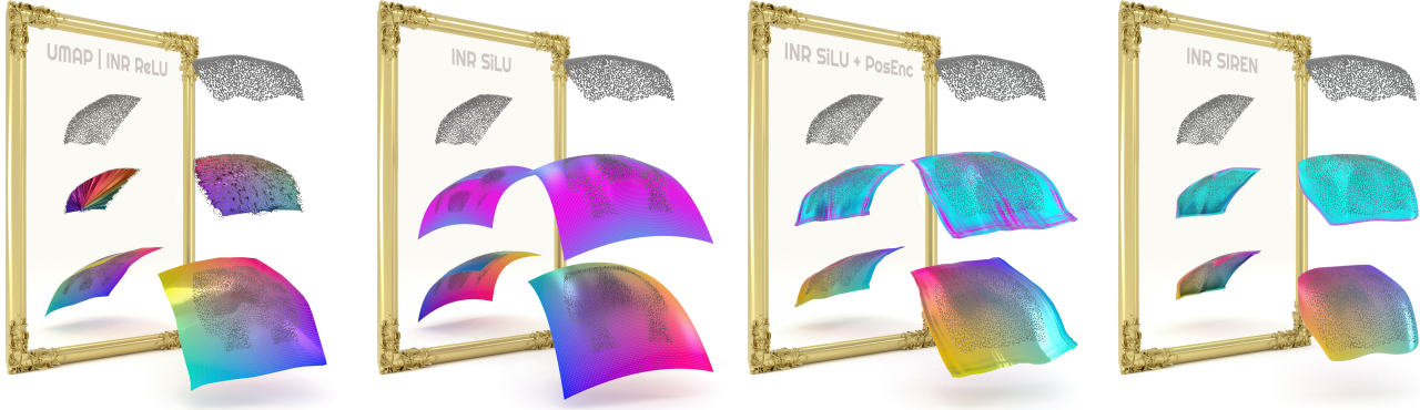
Figure 3. Inspiration items of our INR surface fitting. UMAP [28] (1 st column, middle) learns the underlying 2D manifold of 3D points along with the inverse mapping, but cannot capture its smooth analytic representation. Early experiments with ReLU activations confirmed its low-frequency bias (1 st column, bottom) and piece-wise linearity. SiLU [12] (2 nd column) suffers from low-frequency bias, too. We found that resolving it by adding positional encoding is challenging under our training protocol (3 rd column). SIREN [40] (4 th column) fits the data precisely, however, does not extrapolate well. A combination of the best parts of these ingredients led us to our INR surface fitting method, seen in Fig. 2 and discussed in Sec. 3.2.
