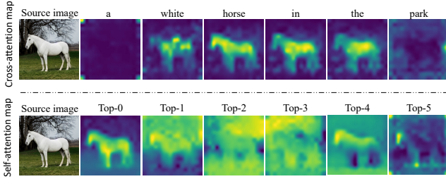
Figure 3. The heatmaps of cross-attention and self-attention maps in a generated image with the prompt "a white horse in the park". The visualization of the cross-attention map corresponds to each word in the prompt. The visualization of the self-attention map is the top-6 components obtained after SVD [36].
