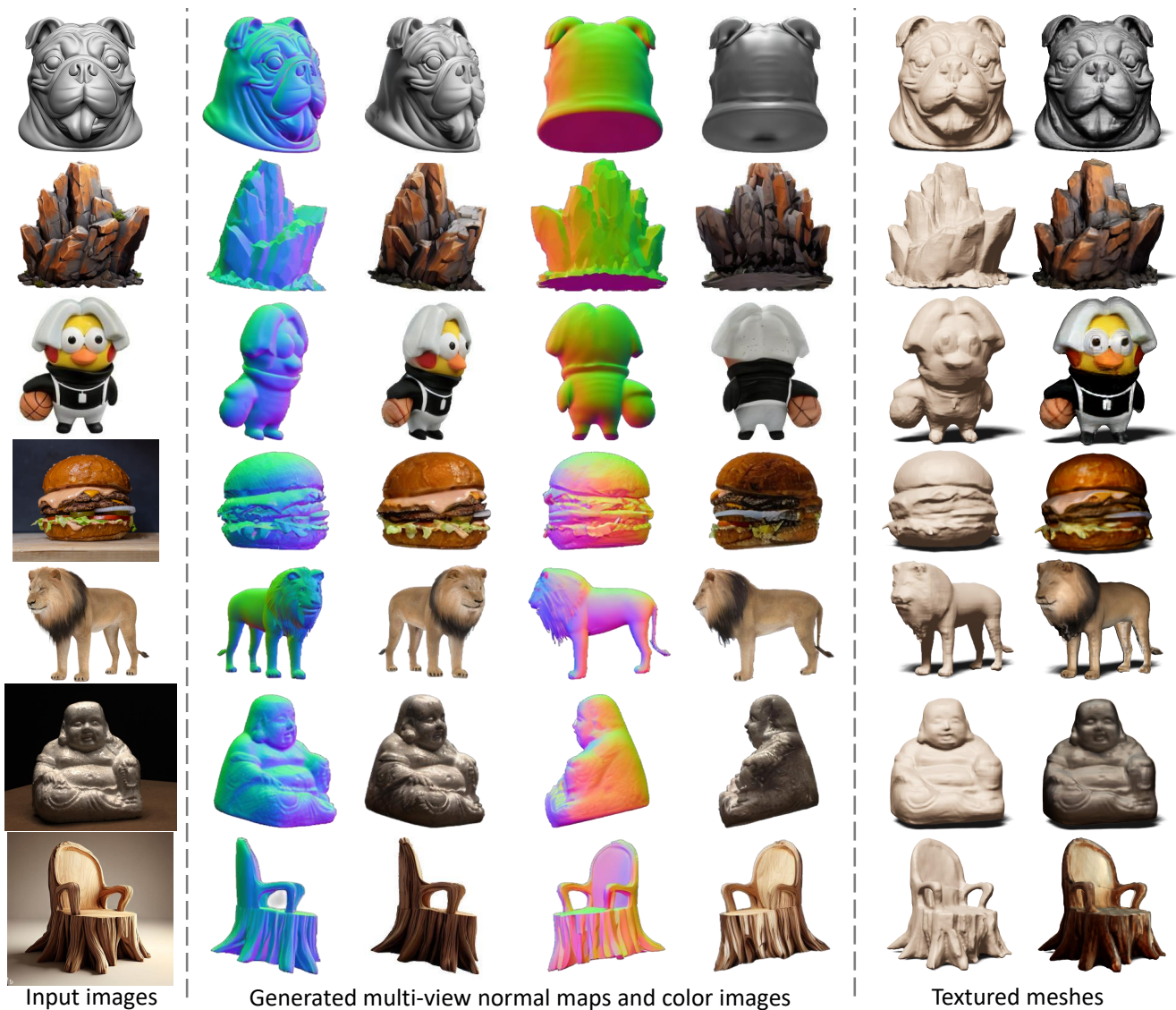
Figure 1. Wonder3D reconstructs highly-detailed textured meshes from a single-view image in only 2 ~ 3 minutes. Wonder3D first generates consistent multi-view normal maps with corresponding color images via a cross-domain diffusion model, and then leverages a novel normal fusion method to achieve fast and high-quality reconstruction. Compared to the prior works, Wonder3D has achieved a leading-level of geometric details with high efficiency.
