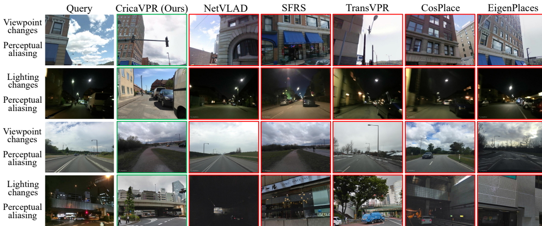
Figure 5. Qualitative results. These four challenging examples show severe viewpoint changes and condition changes. The proposed CricaVPR successfully yields the right results, while other methods return incorrect images. In each example, there are methods to return similar images from different places (i.e., incorrect) due to perceptual aliasing. In the second example, the query image is taken at night, causing all the other methods to return night images but from different places (i.e. wrong). However, our method returns an image taken during the day at the same place (i.e. correct).
