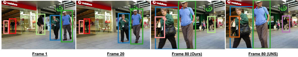
Figure 3. Qualitative comparison between our model and UNS [1]. We visualize the tracking on three frames. UNS cannot track the person in green bounding box once he is occluded and assigns him a new ID (purple) on frame 80. It also fails to track the person in pink bounding box when she is only partially visible in frame 80. We can consistently track with both people with the same IDs (green, pink).
