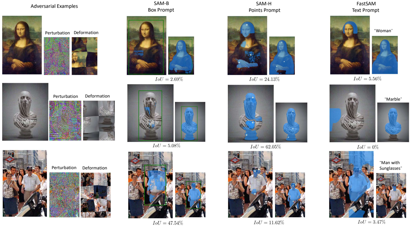
Figure 3. Adversarial examples crafted by our approach. In each row, we present, from left to right: the adversarial example, the adversarial perturbation, the optimized deformation target, attacked segmentation results and the original segmentation results on SAM-B (using a box prompt), SAM-H (using point prompts), and FastSAM (using a text prompt) respectively. The results demonstrate the high effectiveness of our approach against unseen models and versatile prompts.
