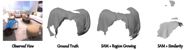
Figure 3. Comparison on different decomposition methods with SAM feature. SAM + region growing represents object extraction with our method. SAM + similarity indicates object extraction with similarity matching in 3D space, following [16, 32].
