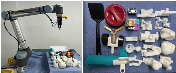
Figure 7. (a) Robotic grasping system and (b) objects for real-world grasping.
