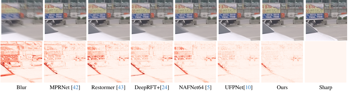
Figure 6. Examples on the GoPro test dataset. The first row shows blur image, predicted images of different methods, and ground-truth sharp image. The second row shows the residual of the blur image / predicted sharp images and the ground-truth sharp image.
