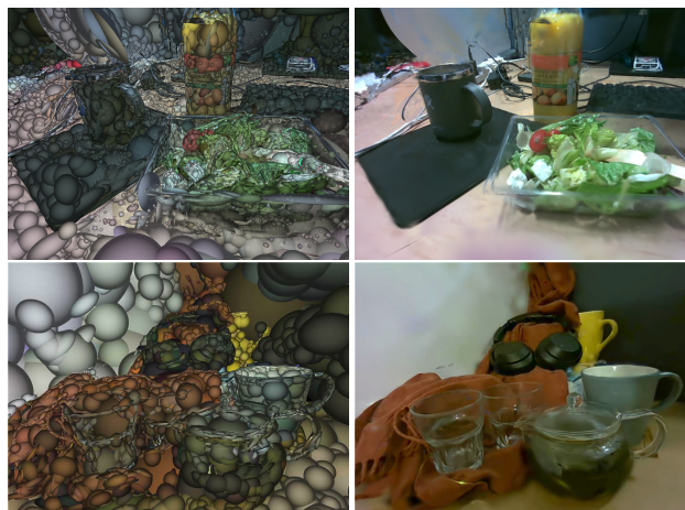
Figure 7. Self-captured Scenes: Challenging scenes and objects, for example, transparent glasses and crinkled texture of salad are captured by our monocular SLAM running live.
