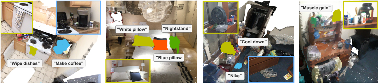
Figure 5. Qualitative results of our method on open-vocabulary instance segmentation. We query instance masks using arbitrary text prompts involving object categories that are not present in the ScanNet200 labels. For each scene, we showcase the instance that has the highest similarity score to the query’s embedding. These visualizations underscore the model’s open-vocabulary capability, as it successfully identifies and segments objects that were never encountered during the training phase of the 3D proposal network.
