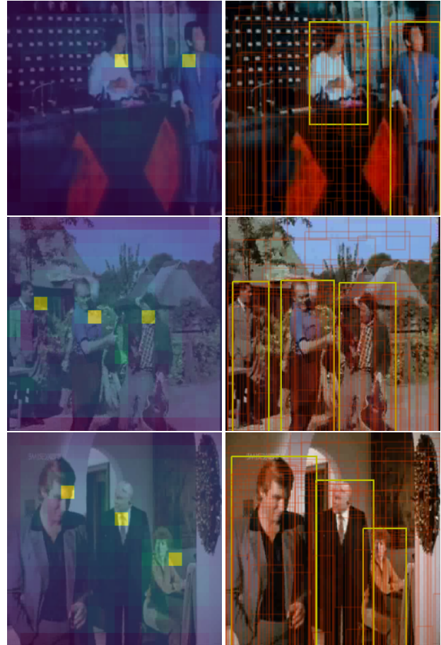
Figure 3. Qualitative analysis. The images on the left show the confidence maps produced by the output 16 \times 16 spatial tokens (rescaled to the image size) w.r.t. the actor likelihood for the corresponding bounding box. For the sake of clarity, we only plot the 256 tokens corresponding to one of the frames. The highlighted tokens are those selected as positive detections. The images on the right show all the bounding boxes computed by the corresponding tokens on the left. We overlay all the bounding boxes returned by each of the 16 \times 16 output tokens. In yellow we represent the bounding boxes corresponding to the confident tokens represented on the left. All other bounding boxes (in red) are assigned to the no-class label \emptyset , and are thus considered as negative predictions
