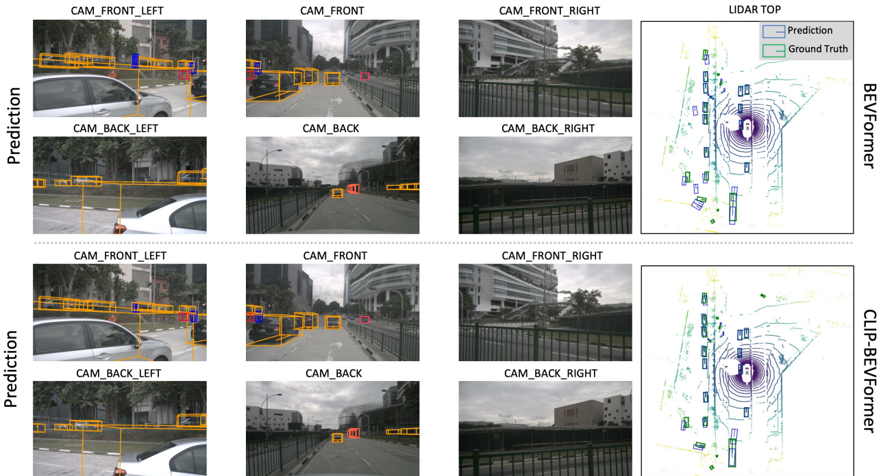
Figure 2. Visualization results on nuScenes validation set. We demonstrate qualitative detection performance on both camera and BEV images. As can be seen in BEV images, CLIP-BEVFormer demonstrates improved alignment with ground truth detections.
