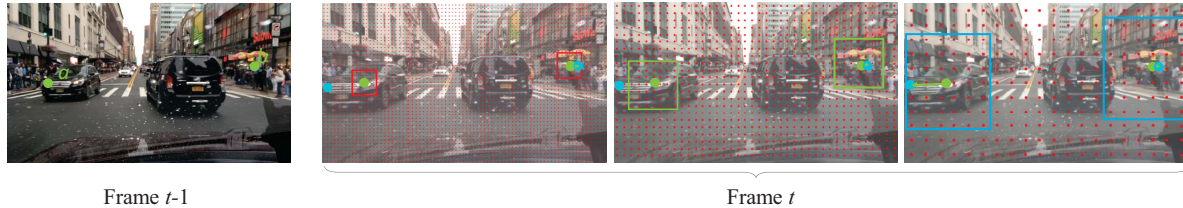
Figure 4. Multi-scale point-region Relation on correlation pyramid. With downsampling, the searching region becomes progressively larger (red, green and blue box). Two examples points a and b are given in the figure, where the green dot and blue dot represent the target point in frame t - 1 and frame t respectively. (a) Headlights of the car. The car moves very fast with large displacement, its relation point in frame t is not captured until the layer with the largest scale (b) Head of the man. Due to the relatively small movement of people, its relation can be obtained at the first level of the pyramid (the highest resolution). Such a relation searching paradigm can be flexibly adapted to both large and small displacements with low computational resources.
