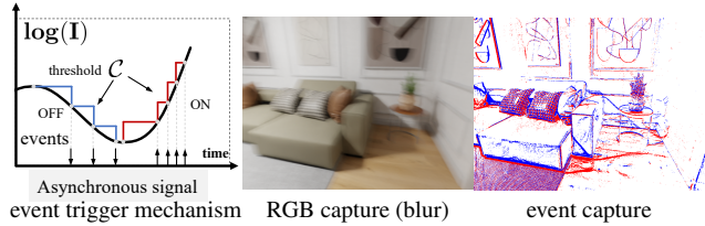
Figure 2. Illustration of the Event Generation Model (EGM). An event is triggered at a single pixel if the corresponding logarithmic change in luminance exceeds a threshold C .
