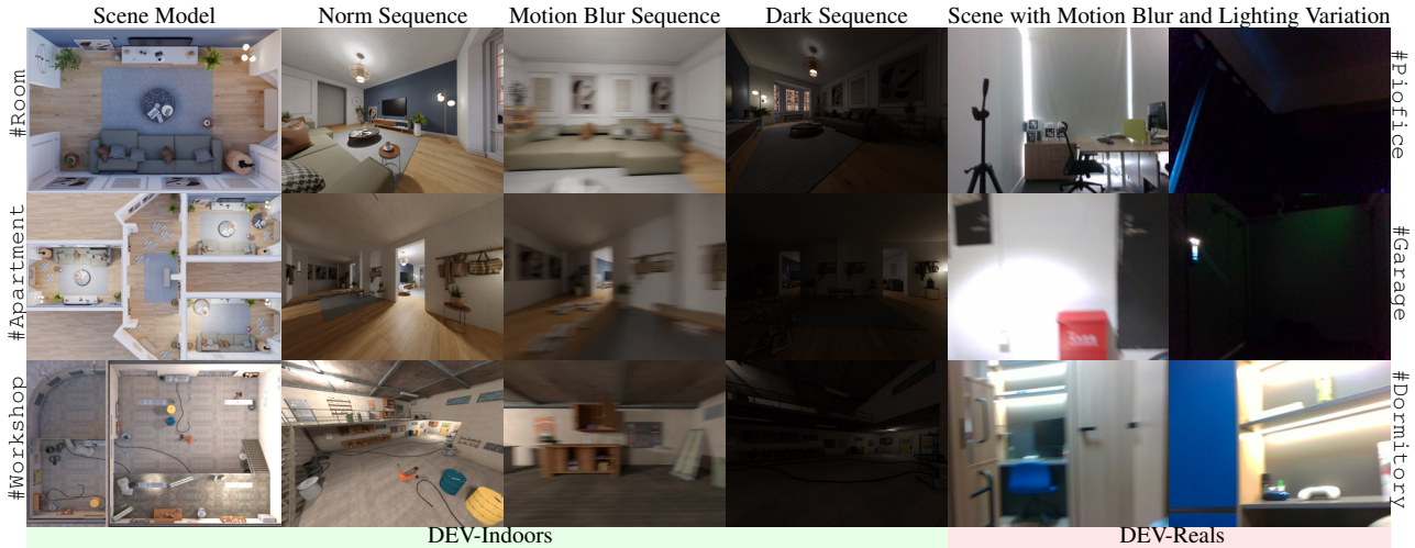
Figure 6. Overview of the DEV-Indoors and DEV-Reals datasets. DEV-Indoors is obtained through Blender [6] and simulator [14], covering normal, motion blur, and dark scenes, providing 9 subsets with RGB images, depth maps, event streams, meshes, and trajectories. DEV-Reals is captured from real scenes, providing 8 challenging subsets under motion blur and lighting variation.
