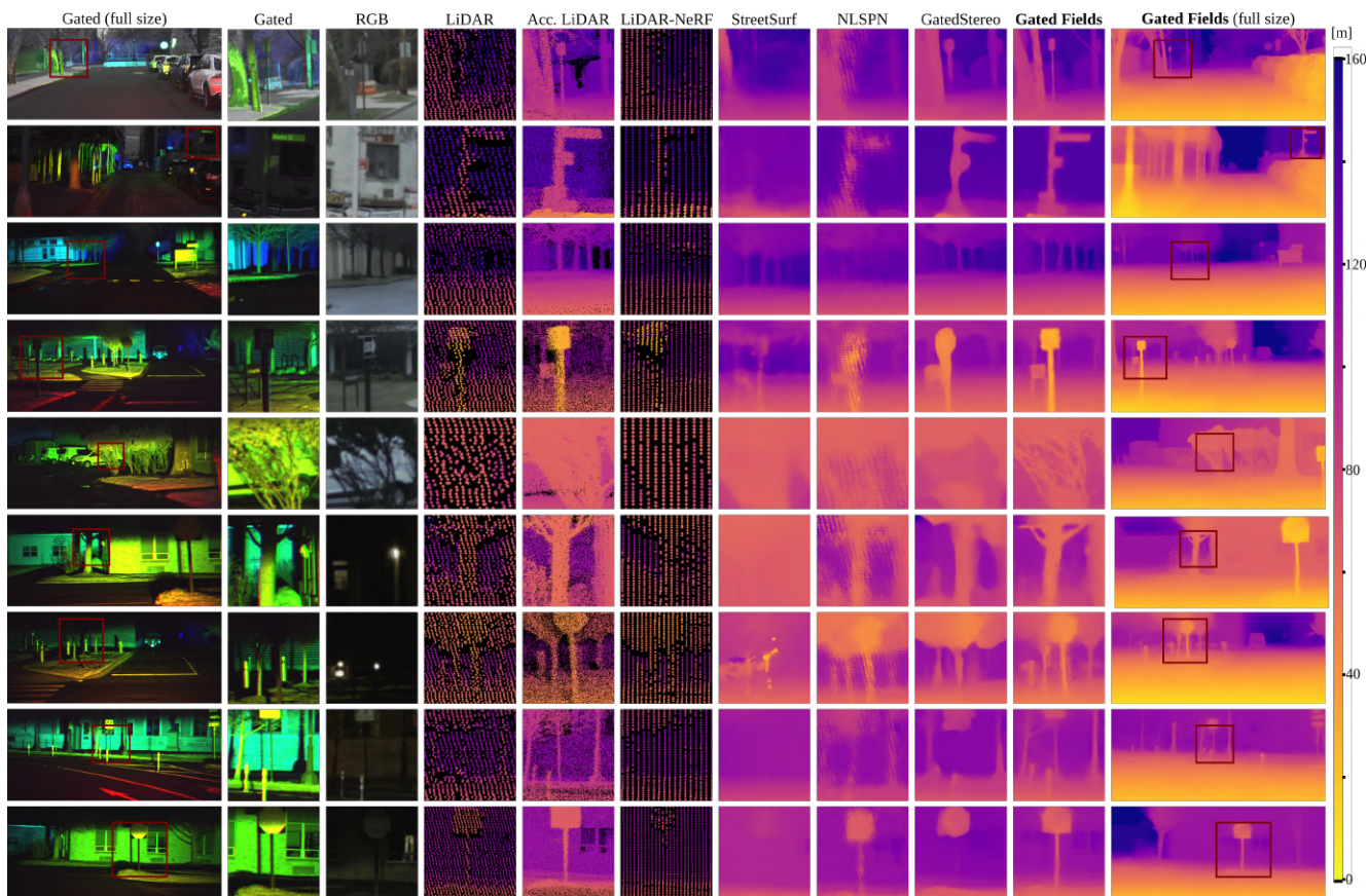
Figure 5. Qualitative comparison of the proposed Gated Fields and state-of-the-art depth estimation approaches, including LiDAR-NeRF [84], StreetSurf [37], NLSPN [67], and Gated Stereo [90]. Compared to baseline methods, we are able to reconstruct fine geometry details like branches or poles, also for far distances. Unlike RGB methods, Gated Fields is unaffected by poor ambient lighting, and unlike LiDAR-based methods it is able to reconstruct sharp object discontinuities. The active gated slices are visualized in red for slice 1, green for slice 2 and blue for slice 3.
