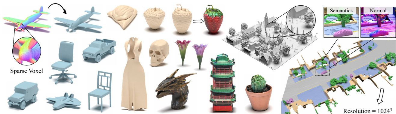
Figure 1. XCube ( \mathcal{X}^3 ). Our model generates high-resolution (up to 1024^3 ) sparse 3D voxel hierarchies of objects and driving scenes in under 30 seconds. The voxels are enriched with arbitrary attributes such as semantics, normals, and TSDF from which mesh could be readily extracted. Here we show randomly sampled geometries using our model trained on ShapeNet, Objaverse, Karton City, and Waymo.
